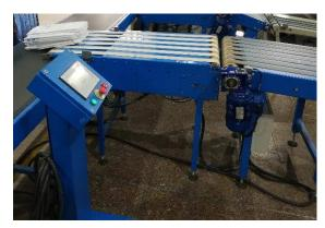
Extensible belts can be activated from the terminal, if installed. They introduce the clothes to the system, in case it is automatic, or are used when it comes to automatic unloading.
